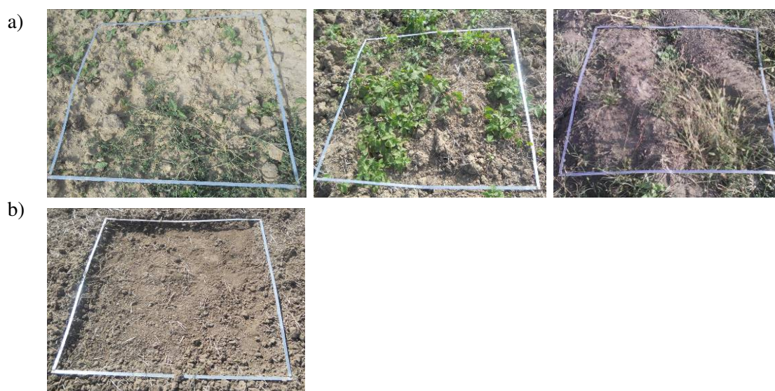
Fig. 8. Aspects regarding determination of coverage degree with plant debris: a – plant debris existing on the soil surface (on 1 m 2 ), before the passage of the tractor-combiner unit; b – plant debris existing on the soil surface (on 1 m 2 ), after the passage of the tractor-combiner unit
